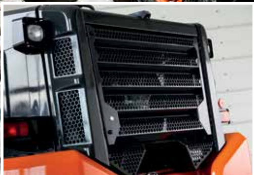
New rear grill protects radiator compartment.
