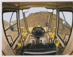
Spacious, comfortable cab (optional): The use a cab with expansive tinted glass relaxes the operator and improves his visibility. Ergonomically arranged instruments, control levers and pedals boost operating efficiency. The cab is mounted on the rear frame with rubber pads to minimize noise and
