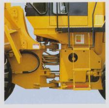
Smooth, light-touch steering: The demand valve system guarantees light-touch steering at all times. An advanced hydraulic design in the steering circuit gives the WA400-1 a smooth steering action and maximizes operator comfort while minimizing soil spillage.
