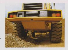
High machine stability: A centerpin-supported rear axle and large oscillation angle maintain level operation on even the roughest surfaces. This, plus a long wheelbase, wide tread and large static tipping load, give the WA400-1 high stability for efficient digging/ carrying operations.
