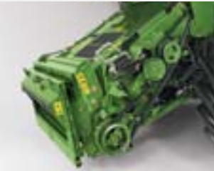
Heavy duty Feederhouse Drive The durable high-torque slip clutch ensures peak performance and a long lifecycle.
