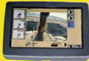
The integrated video functionality in the GreenStar 3 Display allows a perfect view to the rear of the combine, in the grain tank or on the unloading auger – providing excellent, customizable views, when having a camera installed.
