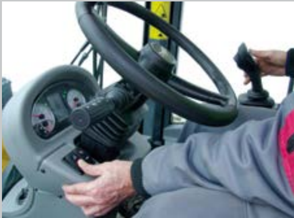
Electrical proportional adjustment of the hydraulic performance of the 3rd and 4th circuits.
