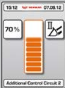
Electrical proportional adjustment of the hydraulic performance of the 3rd and 4th circuits.
