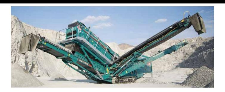
The Powerscreen® Chieftain 1700 is a mid-sized track mobile screen aimed at end users requiring high volumes of finished products in applications including topsoil, coal, crushed stone, recycling, iron ore, sand and gravel.
