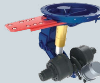
+ Goldhofer pendular axle with ball bearing race ring
