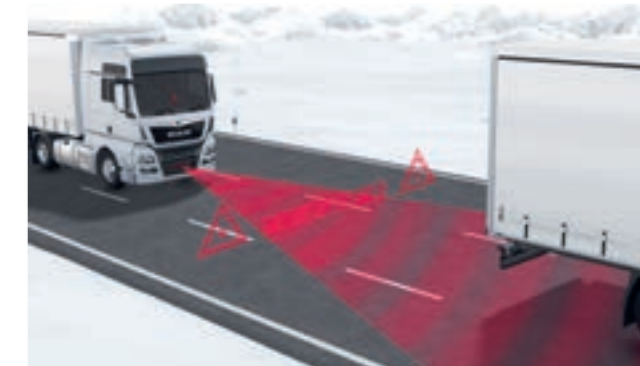
Functional principle EBA: advanced traffic monitoring by using two independent sensor systems (radar and video)
