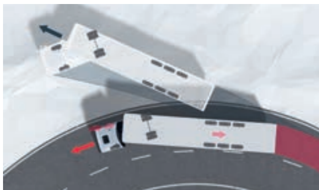
ESP compensatory braking when vehicle is oversteered
