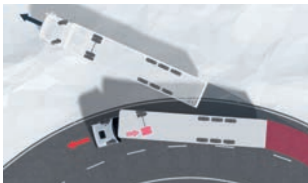
ESP compensatory braking when vehicle is understeered
