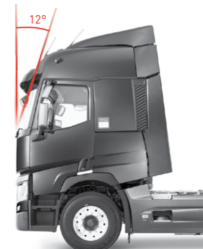
12° INCLINED WINDSCREEN for a better aerodynamic profile.
