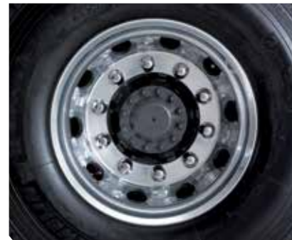
ALUMINIUM WHEEL RIMS reduce the weight of the vehicle by up to 200 kg.
