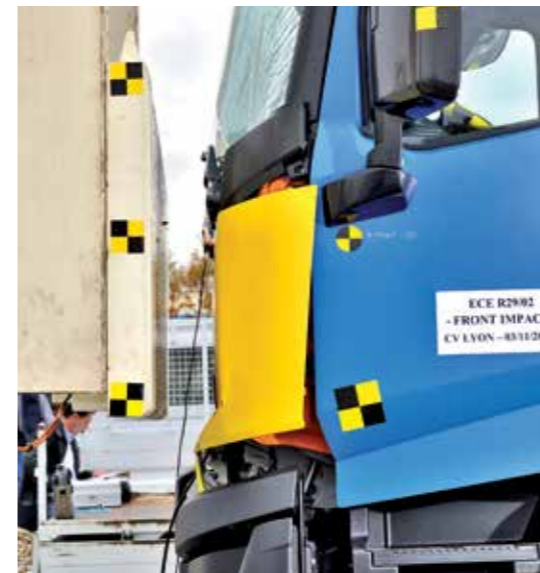
FRONTAL IMPACT to measure the cab impact resistance.
