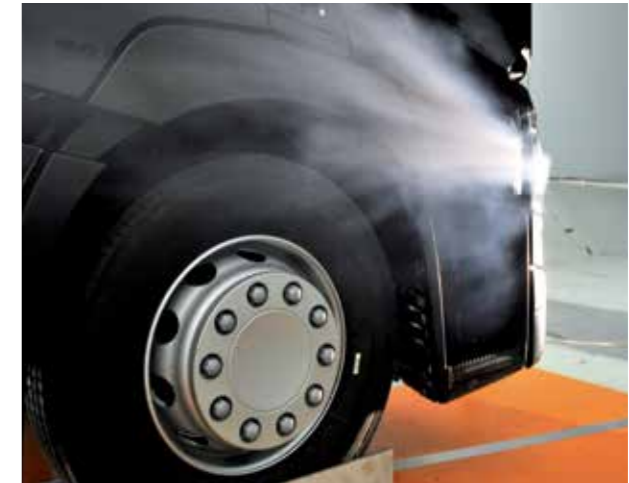
WIND TUNNEL to measure cab air flow resistance.
