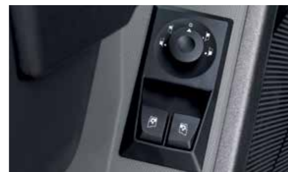
MANAGEMENT OF SIDE WINDOWS AND MIRRORS one-touch window lift and electrically adjusted main and wide-angle rearview mirrors.
