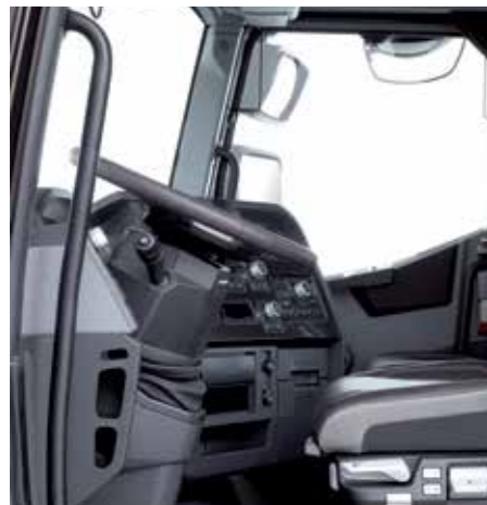
STEERING WHEEL ADJUSTABLE IN THREE DIMENSIONS height, depth, rake.
