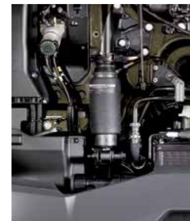
CAB AIR OR MECHANICAL FRONT SUSPENSION suitable for heavy-duty use for improved vehicle stability.
