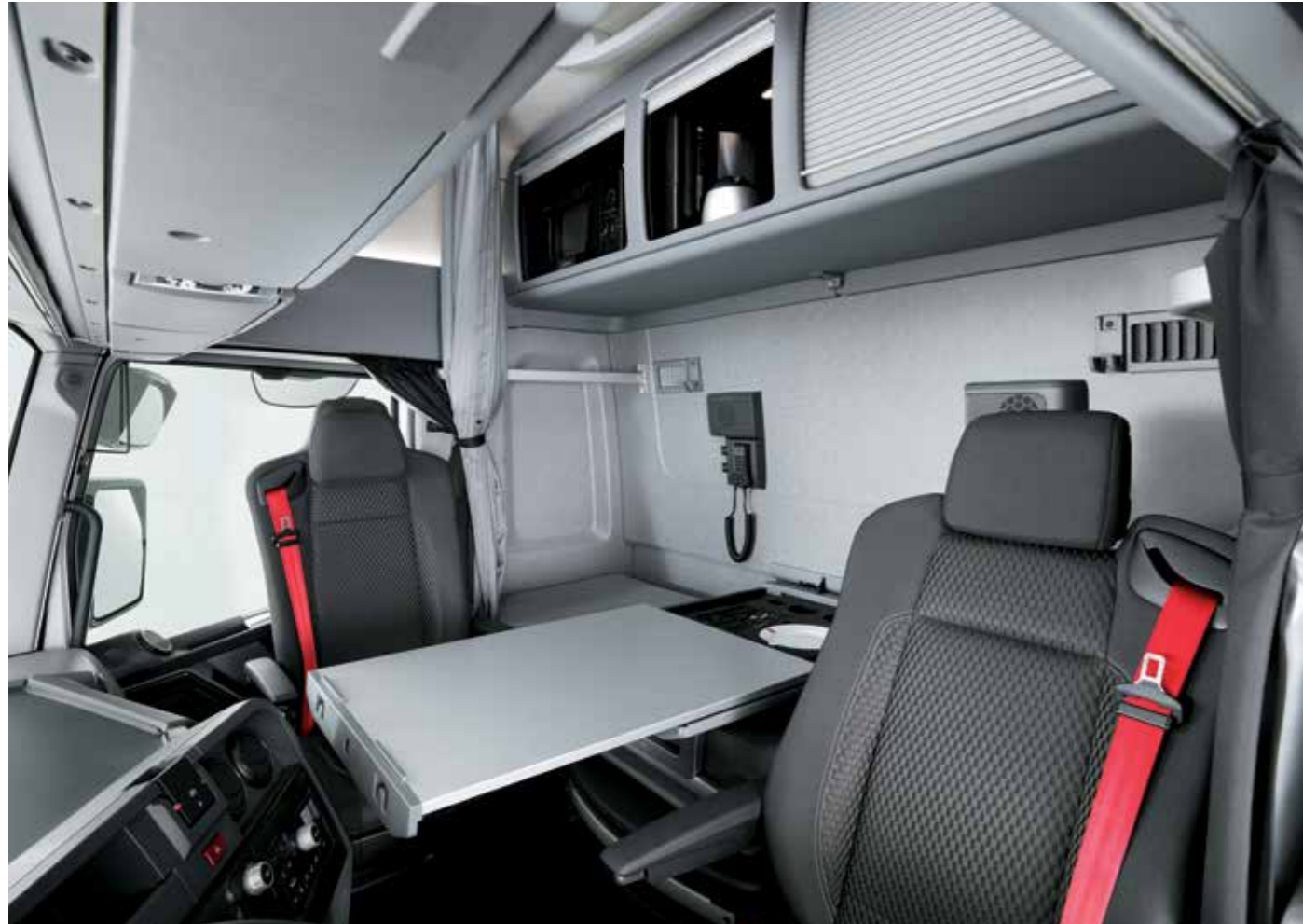
MAXISPACE CAB ARRANGEMENT with a fold-up shelf and additional storage console at the rear of the cab comprising three storage compartments.
