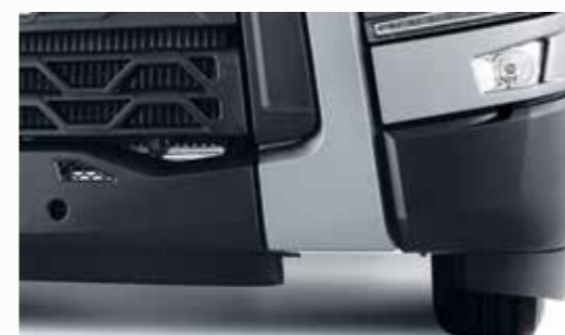
AERODYNAMIC BUMPER EXTENSIONS to improve air penetration.
