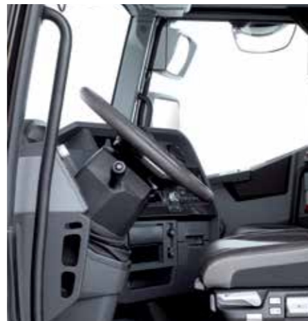
STEERING WHEEL ADJUSTABLE IN THREE DIMENSIONS height, depth, rake.
