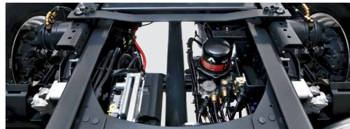
SEPARATION OF WIRING HARNESSES AND AIR HOSE BUNDLES for easier maintenance.
