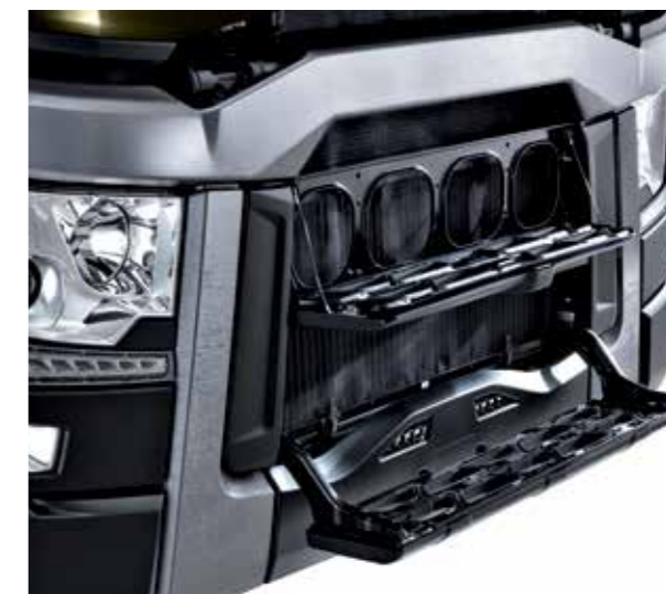
ACCESS TO THE WINDSCREEN via two platforms for cleaning the windscreen.
