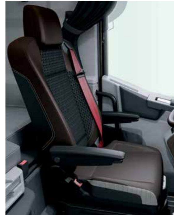
HEATED, VENTILATED SUSPENDED SEATS with integrated seat-belts headrest, adjustable side and lumbar supports. Pushes back 20 cm for added leg-room.
