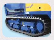
• A heavy duty rubber track undercarriage and chassis reduce impact on the ground with balanced weight distribution. Four sea-saw type rollers maintain a comfortable, even ride even in difficult terrain as well as help absorb shock to the undercarriage and keep maintenance costs down.
