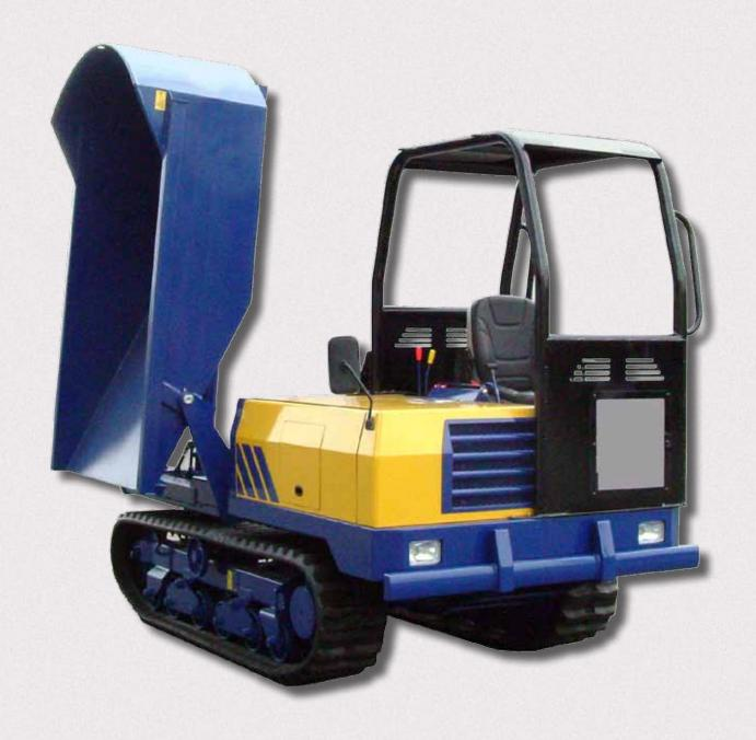
The Canycom S25A Heavy-duty Carrier with 180° Pivoting Dump Box is designed for excellent performance and precise maneuverability in extreme conditions. The 46 HP Kubota Diesel engine hauls up to 5510 LBS and climbs grades up to 25° with ease.
