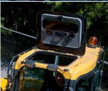
Opening skylight for overhead visibility
