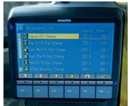
The LCD monitor informs about abnormalities and replacement times
