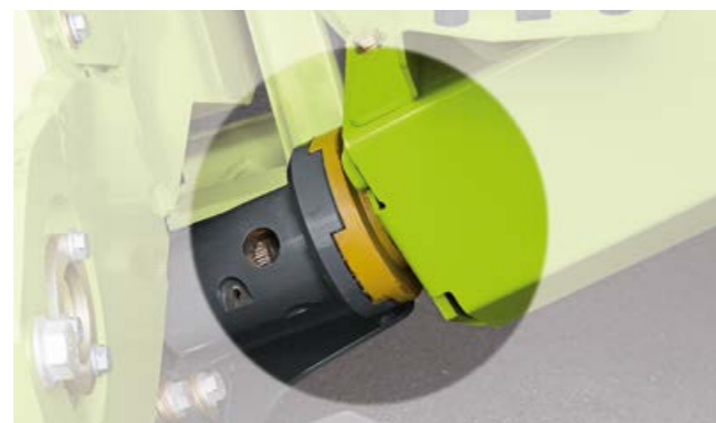
Power transmission via quick release coupler
