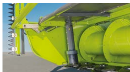
Adjustable roller crop press bars, optionally with hydraulic operation
