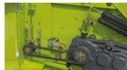
DIRECT DISC 600 P / 500 P: adjustment of paddle roller height, optional hydraulic adjustment also available
