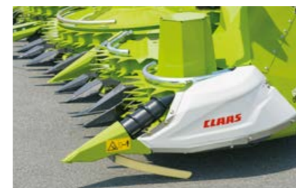
Lodged maize point hydraulically driven
