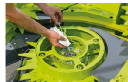
Dipstick to check oil level
