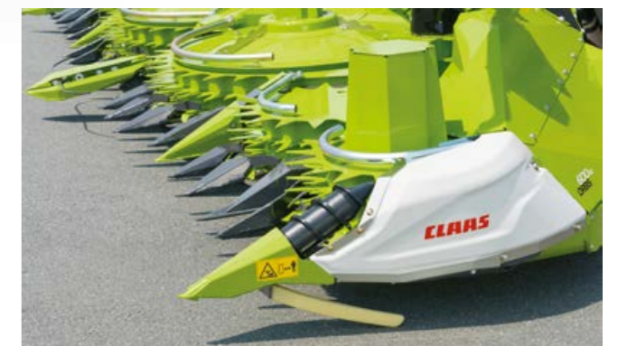
Where necessary, the lodged maize augers are driven hydraulically
