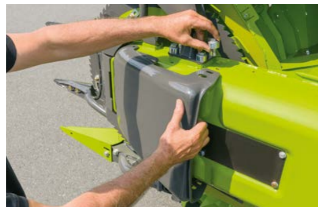
Sliding skid with two height settings
