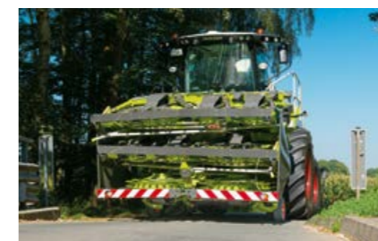
ORBIS 900 with 3.3 m transport width
