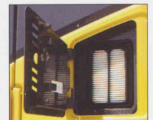
External air conditioner filter
