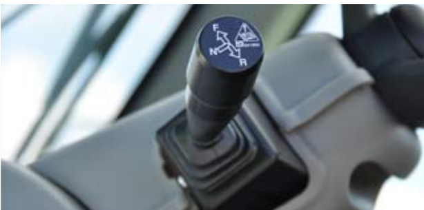
▲ A column-mounted Finger-Touch electrical control lever allows the driver to reverse driving direction without taking his hands off the steering wheel.
