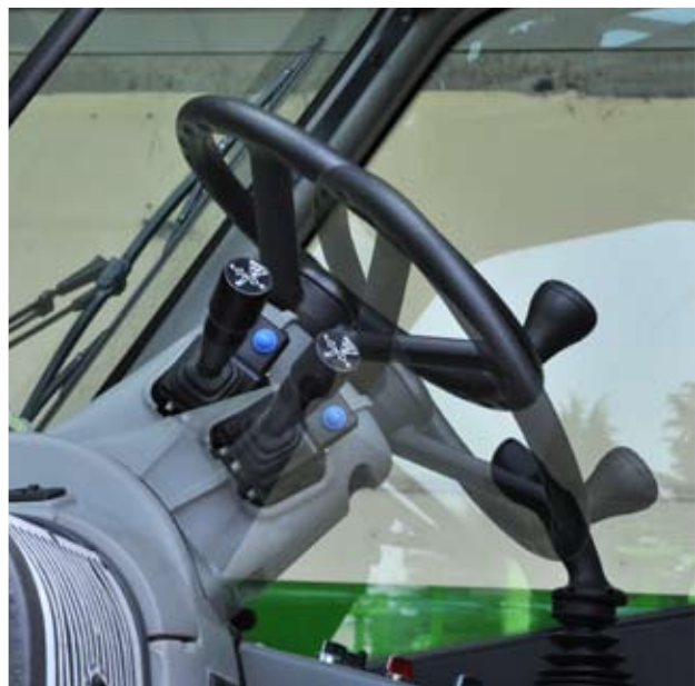
▲ A column-mounted Finger-Touch electrical control lever allows the driver to reverse driving direction without taking his hands off the steering wheel.
