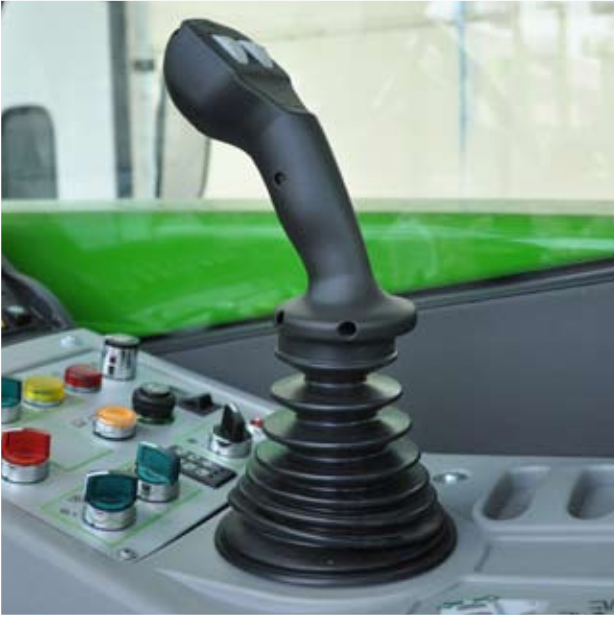
▶▶ The standard Inching Control , operated either by a pedal or a multi-turn potentiometer , ensures minute control of the machine while maintaining a high engine speed; this feature is highly productive while excavating and stockpiling materials. The high/low travel speed range selector is electrically operated. A Shift-on-the-Go gearbox with electronic synchronization is available as an option.
