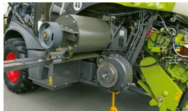
Straightforward removal and installation of the accelerator
