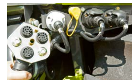
Quick coupling adaptation for maize pickers
