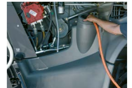
Additive tank with capacity of up to 375 l.
