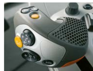
CMOTION multifunction control lever
