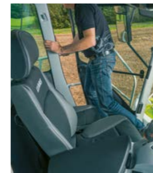
Seat contact switch: front attachment and main drive are switched off automatically
