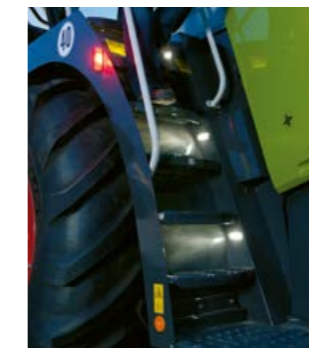
LED step lighting
