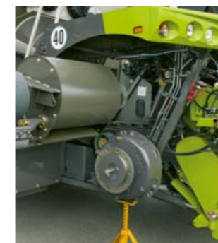
Quick removal of accelerator
