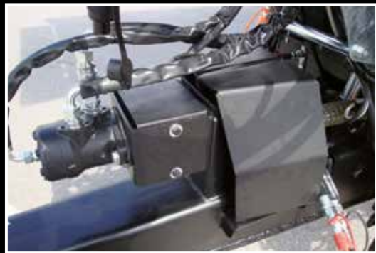
Ribaltamento pompa / motore Omhoog hydro / pomp Tilting motor / pump Bennage pompe / moteur hydraulique kippping pump / motor
