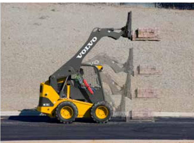
Parallel-lift (attachment remains parallel to the ground throughout the raise cycle)
