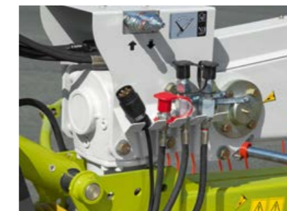
Hydraulic sequential control fitted as standard to adjust the time delay between front and rear rotors when raising and lowering.
