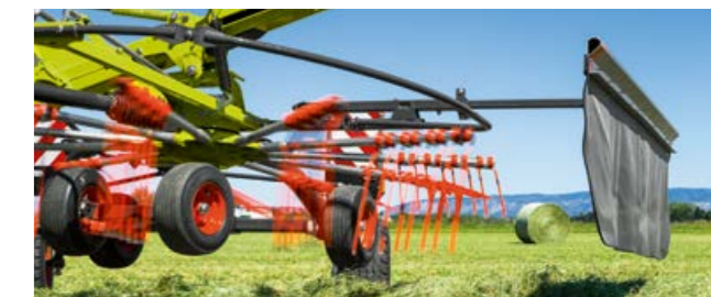
The unique chassis design of the CLAAS side swather allows lift heights of up to 70 cm.
