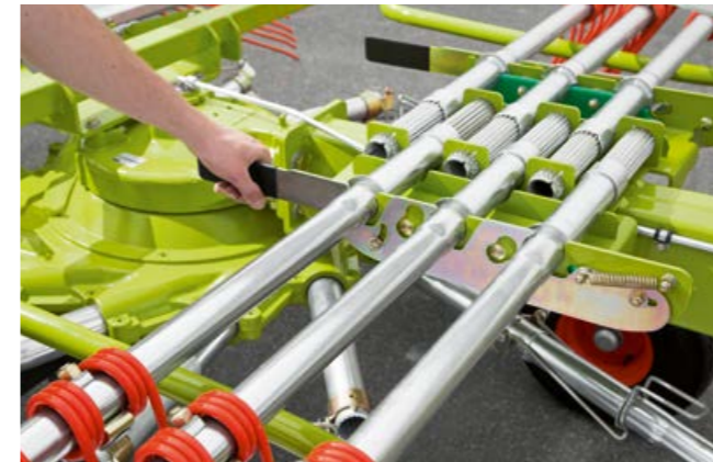
For some models, the tine arms have to be removed for road transport – but they can be stowed away in no time at all.
