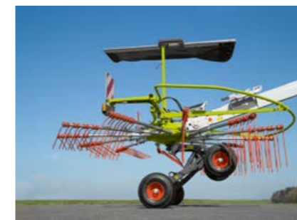
Generous lifting height for driving over swaths at headlands: up to 50 cm in the LINER 700 TWIN.
