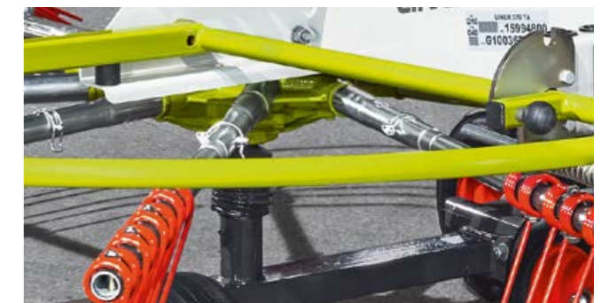
Lemon profile attachment and clamping splint in the LINER 370 and 320.
