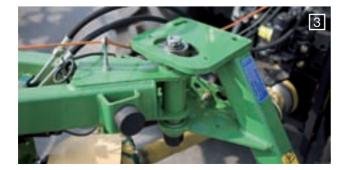
driveshaft on the pivoting headstock make for tightest headland turns.
