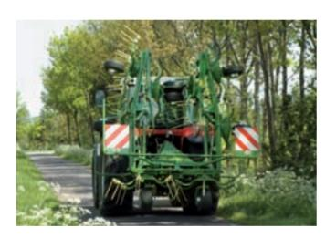
Safe travel on the road KW 8.82/8 folds into a compact transport unit 3.45 m (11'4") high and 2.85 m (9'4") wide, making road travel a safe and relaxed affair.
