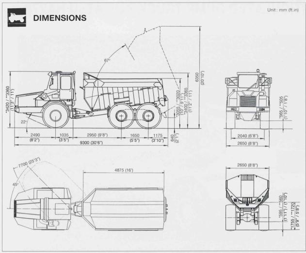
Note: \*dimensions for unloaded / \*\*dimensions for loaded
