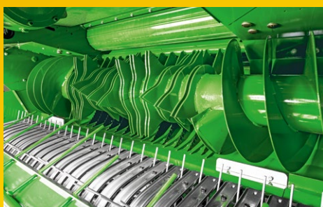
MaxiCut HC is available with either 13 or 25 knives.
