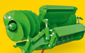
The drop floor provides hands-free unplugging.
