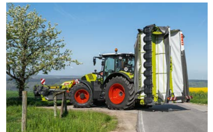
Less than 4.0 m high, and a compact package all round, like all DISCO models. The two mowers retract telescopically, and the machine then folds into the road transport position.
