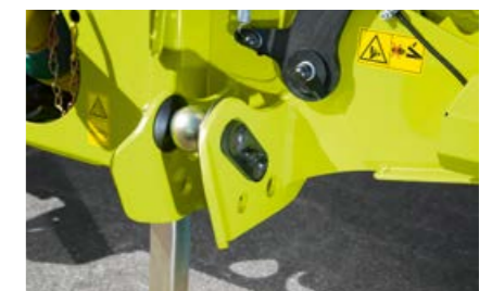
Lower link guide clips for ease of mounting.
