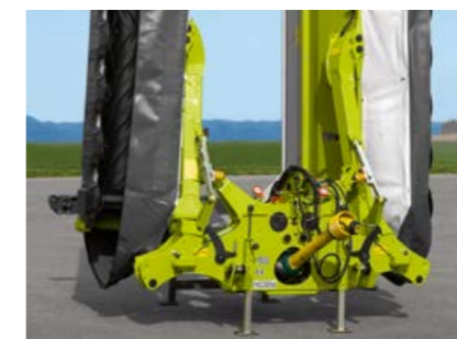
Space-saving: stable parking position for all large-scale mowers.
