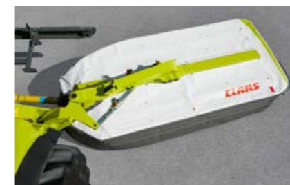
Mechanical breakback protection: in the event of a collision, the machine is moved back and slightly upwards (hydraulic nonstop breakback protection in the DISCO 1100 TREND).
