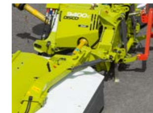
Hydraulic non-stop breakback protection in case of a collision impact – the mower pivots, and is automatically placed in the starting position.
