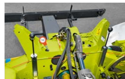
Pressure-gauge dial to conveniently set the ground pressure for both mowing units.
