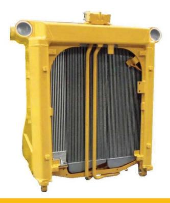
The D6T cooling system is durable and efficient, utilizing aluminum bar plate construction on the radiator cores and Air To Air After Cooler (ATAAC). Aluminum bar plate provides durability and allows for high heat transfer and superior corrosion resistance. The radiator consists of twin unit cores that act together as one heat exchanger.
