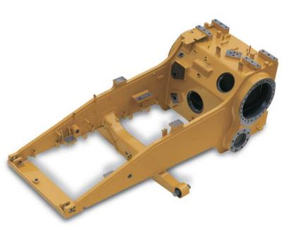
The foundation of every Cat dozer is a rugged frame built to absorb high impact shock loads and twisting forces. A reinforced saddle, welded front cross-member and steel castings on the main case add to the overall strength.
