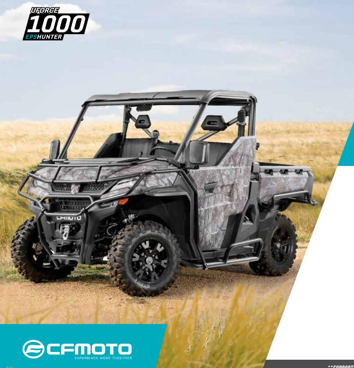
• 71 HORSEPOWER CFMOTO 1000CC V-TWIN ENGINE CANADIAN CVTECH TRANSMISSION • 2WD/4WD AND A LOCKING FRONT DIFFERENTIAL • REAR LIMITED SLIP DIFFERENTIAL (LSD) • ELECTRONIC POWER STEERING (EPS)
