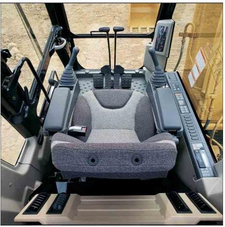
**Viewing.** Window glass is affixed directly to the cab, eliminating window frames which interfere with the operator's viewing area. A larger right-side window also enhances viewing.
