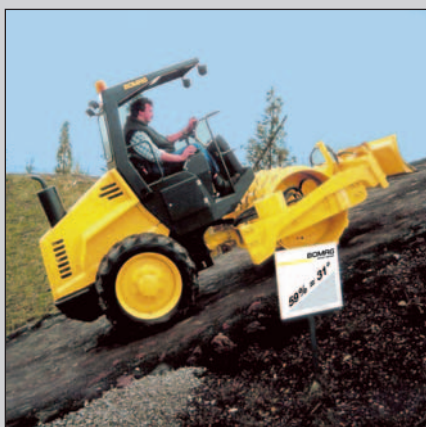
With or without vibration, the BW 124 attains a gradability of more than 55 %.
