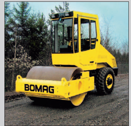
The BW 145 compacting a frost layer in road construction.
