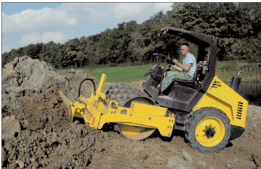
A BW 124 PDH-3 with swivel blade shapes the surface on a golf course.
