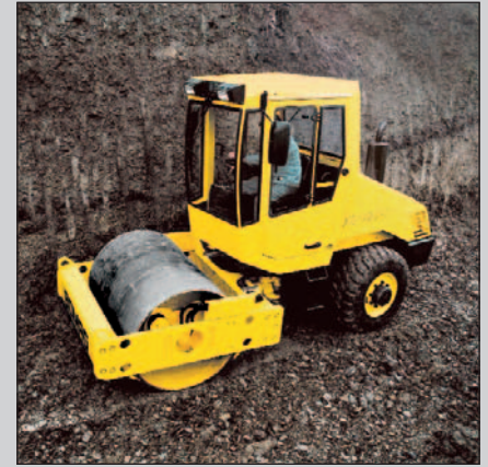
Single drum roller BW 145 D-3 compacting backfill.
