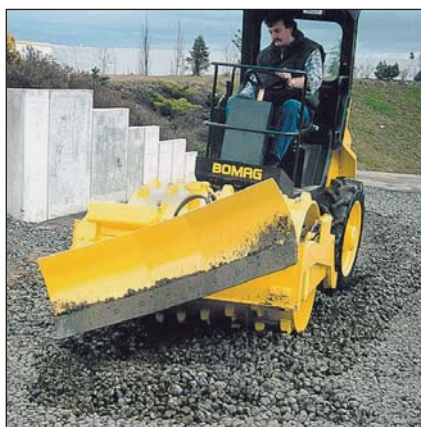
BW 124 with tilting blade.
