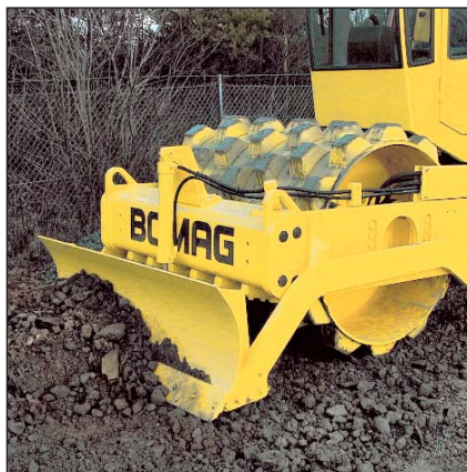
BW 145 with optional blade with "Up" and "Down" function.
