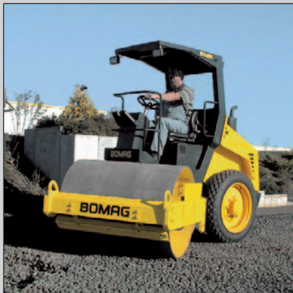
BW 124 DH-3 compacting crushed material.
