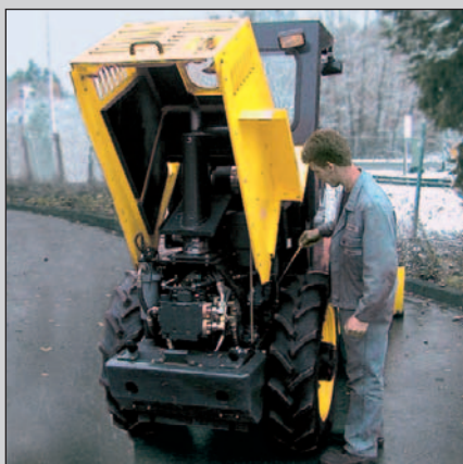
With the engine hood open daily maintenance work is carried out comfortably from one position.
