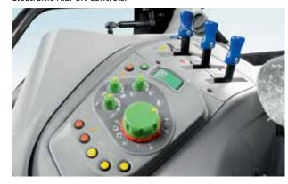
Mechanical rear lift controls.
