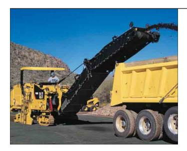
**Hydraulic folding conveyor.** Machine transportation is made easier by the upward hydraulically folding front conveyor that reduces the machine dimensions.
