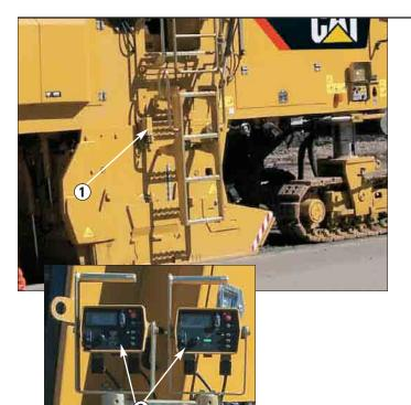
**Contact or non-contact grade sensors.** Sensors can be easily positioned on each side of the machine and provide a consistent accuracy. Cross-slope sensor adds to system versatility.
