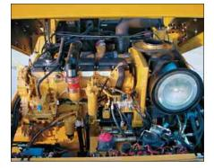
The power-assist engine hood opens wide to provide optimum access to the engine, air filter, hydraulic components and daily service points.
