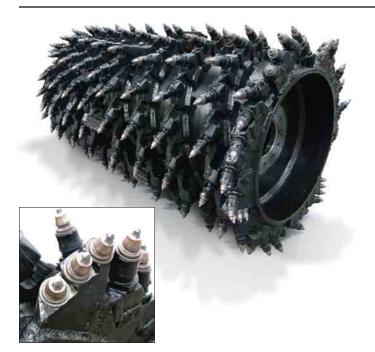
**178** six-sided carbide-tipped tools. Tools are mounted in durable three-piece, quick release tool holders and arranged in a triple wrap flighting pattern for maximum breakout force. Tapered quick release conical tool holders maintain tightness in holder base.
