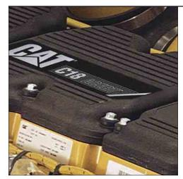
**Optimum power.** The engine performs at a full-rated gross power of 429 kW (583 hp) at 1900 rpm with a torque of 2718 Nm. The combination of large displacement and high torque allow the PM200 to achieve maximum production. Engine power curve is optimized for milling applications providing optimum power while keeping the engine operating at peak efficiency.
