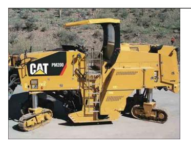
**Four steering modes.** Steering control provides four steering modes for maneuvering in tight quarters: front steer, crab steer, coordinated steer and rear steer.
