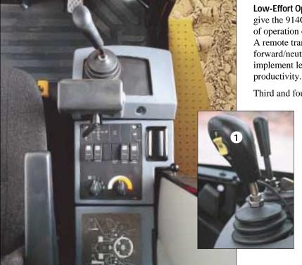
Low-Effort Operation. New pilot hydraulic controls give the 914G uncompromised ease of operation of lift, tilt, and quick coupler functions. A remote transmission control option adds a forward/neutral/reverse control switch (1) on the implement lever for easier operation and enhanced productivity.
