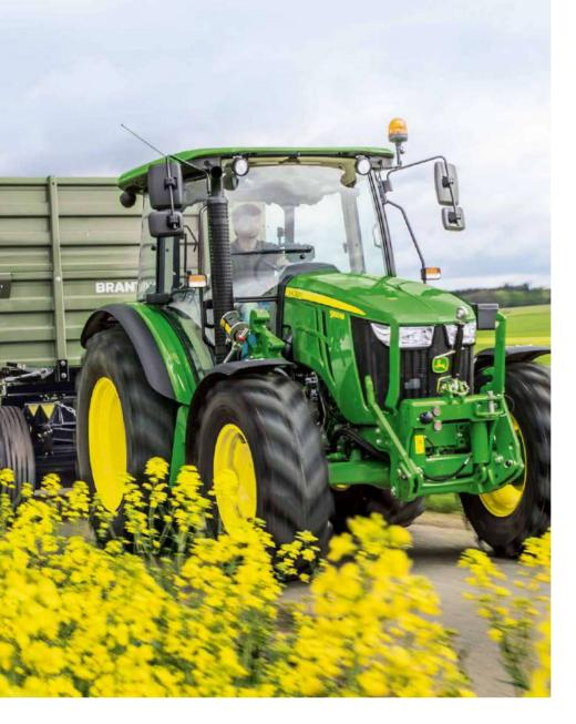
No additives required. By combining cooled Exhaust Gas Recirculation (EGR) technology with an intercooler and Diesel Particle Filter (DPF), iT4 emissions standards are met without the need for any additives.
