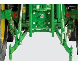
Hook up whatever you need for the job. Built to handle even the heaviest of implements, the super robust rear hitch of the 5M iT4 has  $\dot{a}$  maximum lift capacity of up to 4,330 kg (maximum lift capacity at hooks).
