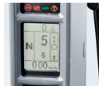
The Power-8 display integrated into the A-post instrument panel. Is well within the operator's field of vision and indicates selected gear, travel direction, Easy Tronic and Steyr Matik modes.
