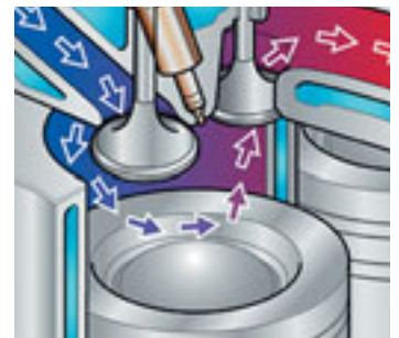
Efficient cross-flow cylinder head design for maximum performance.
