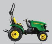
Wheelbase - 63 in. (1600 mm) (2320) 65.2 in. (1655 mm) (2520, 2720)
