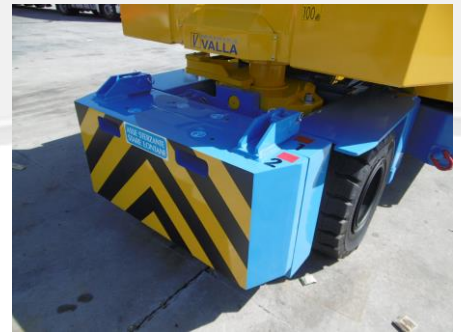
Removable counter (3450 kg) to facilitate the crane's transport
